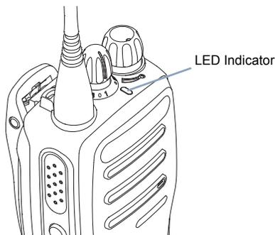
*The LED lights up solid green while the radio is transmitting and blinks when the radio is receiving.*
