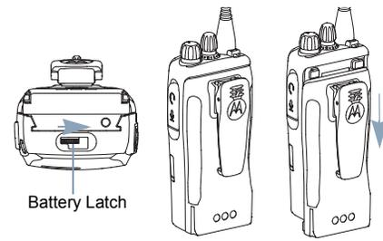
*To remove the battery, turn the radio off. Move the battery latch into unlock position and hold. Slide the battery down and lift off the rails.*
