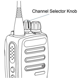
Use the Channel Selector Knob to switch between an analog or a digital channel.
