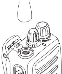
With the radio turned off, set the antenna in its receptacle and turn clockwise.
