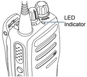
**Blinking red** – Radio is transmitting at low battery condition, receiving an emergency transmission or has failed the self-test upon powering up, or has moved out of range if radio is configured with Auto-Range Transponder System.
