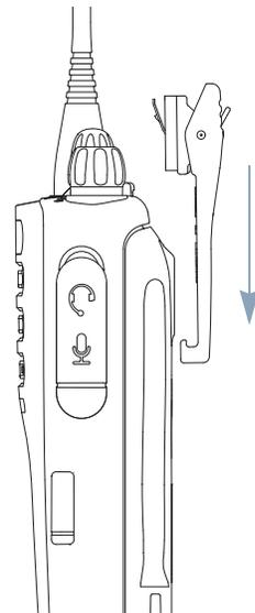
Align the grooves on the clip with those on the battery and press downwards until you hear a click.
